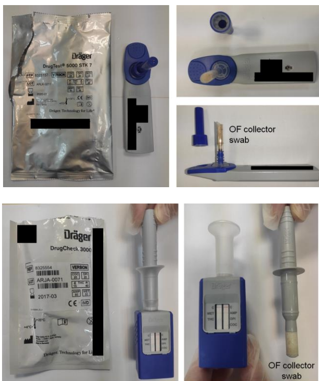
Figure 1: Technical on-site devices for OF screening of drugged drivers a. Dräger DrugTest 5000 and b. Dräger DrugCheck 3000.
