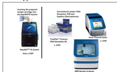
Figure 2 Rapid DNA System and Conventional System Analysis Steps in Forensic DNA Analysis
